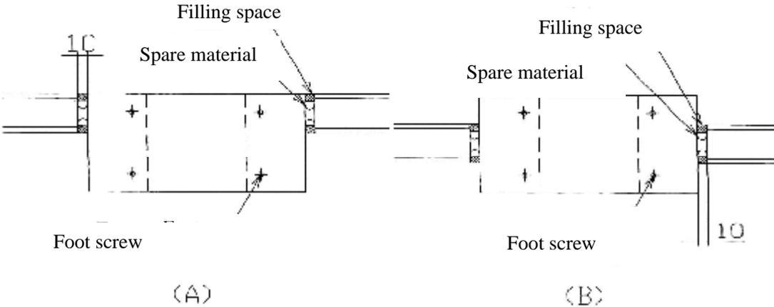
③ Processing for fixing bottom of the body
