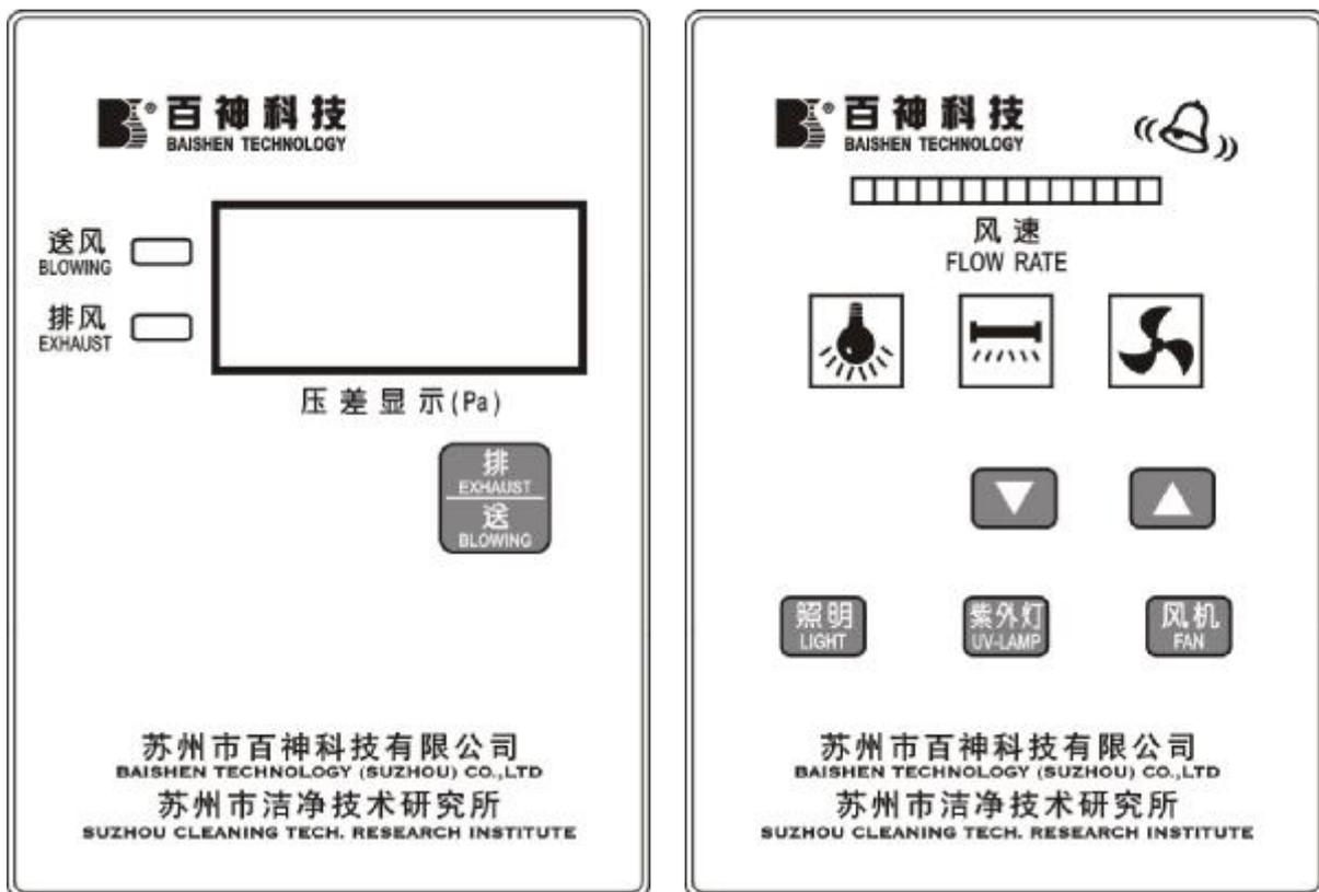
6.1 Turn on the power supply: insert the power cord plug into the socket of the equipment rear, insert another end to the power socket, open the switch with the key, the screen of differential pressure turns to red, indicate the power is on.
